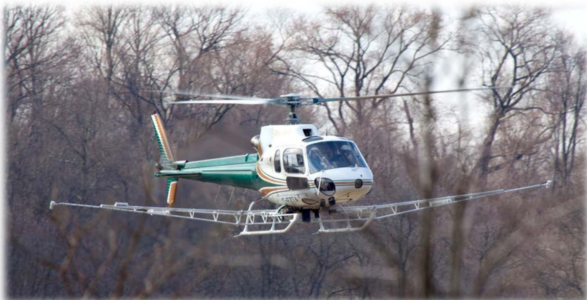
Figure 7. Helicopter magnetic survey of the Washington County Marcellus Site. Pilot flew as close to the ground as possible to maximize the magnetic response of wells.
