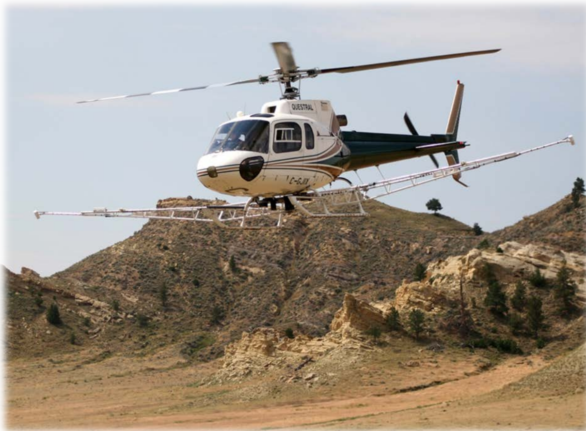
Figure 2. Helicopter magnetic survey to locate oil and gas wells at Teapot Dome Oilfield (Naval Petroleum Reserve No. 3) near Midwest, Wyoming
