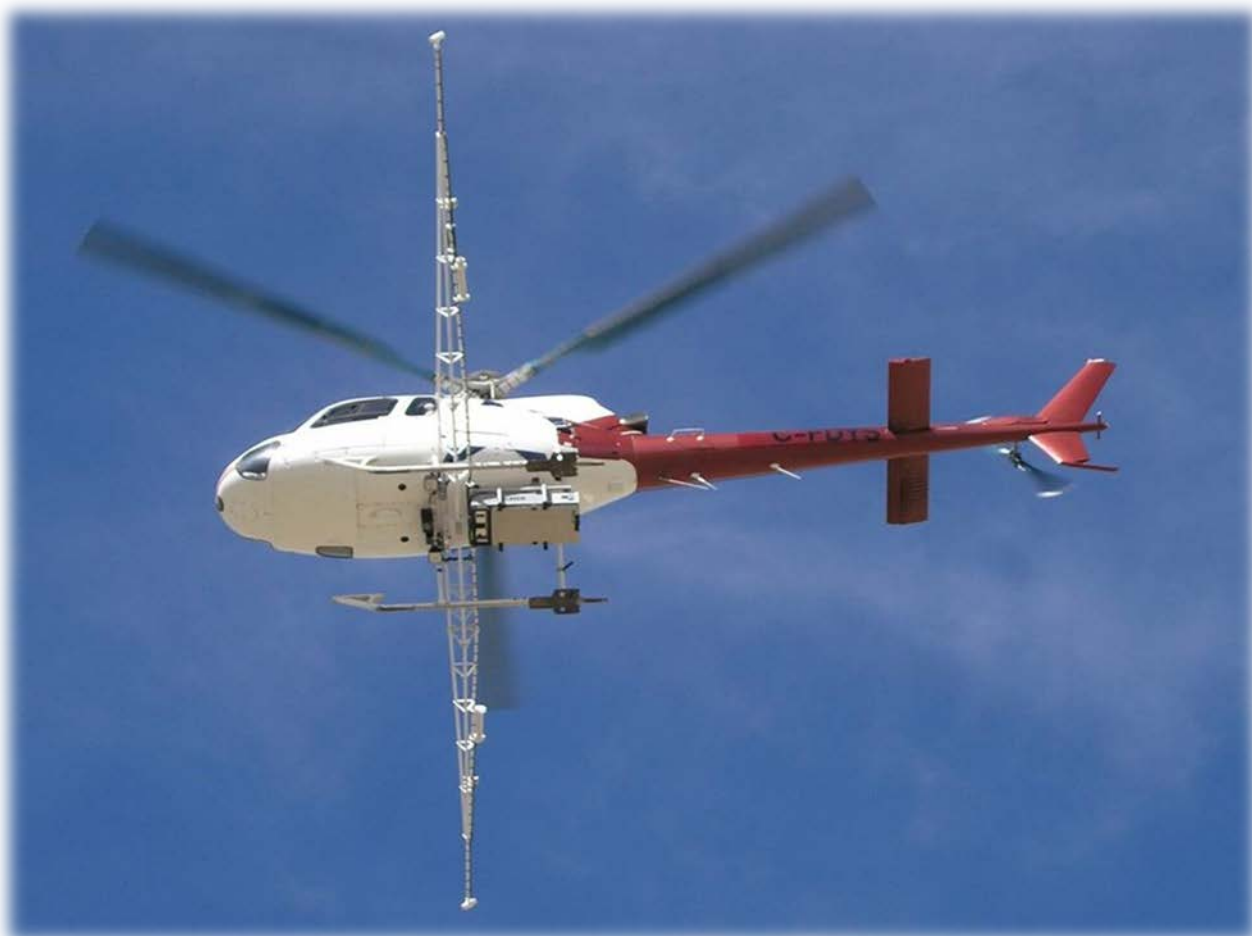
Figure 1. A helicopter with two, boom-mounted magnetic sensors was used to detect well-type magnetic anomalies at the Salt Creek Oilfield in Wyoming. The instrument mounted under the aircraft (between the skids) is a differential absorption LiDAR (DIAL) sensor that detects methane in the air column below the aircraft.
