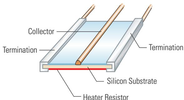
Fig. 3 Chip-type Sensor
