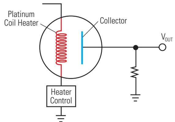
Fig. 2. Schematic Diagram of a Bead-type Sensor
