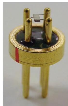
*Fig. 1 A solid-state sensor used for detecting more than a hundred toxic gases.*
